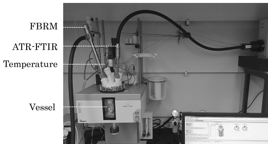
Figure 4.2: OptiMax system from Mettler Toledo equipped with probes for focused beam reflectance measurements (FBRM) and attenuated total reflectance Fourier transform infrared (ATR-FTIR) measurements.
